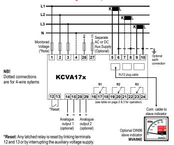
NB! To ensure correct kVAr measurement, the voltage phase sequence and CT connections must be as shown on connection diagrams.
