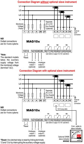
12 and 13 or by interrupting the auxiliary voltage supply. NB! To ensure correct kW measurement, the voltage phase sequence and CT connections must be as shown on connection diagrams.
