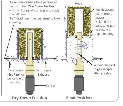
The SADP*mini*-Ex has been specifically designed to be Intrinsically Safe in hazardous environments and because of this it can be used in a wide range of applications including natural gas production, petrochemical production and explosive gases.
