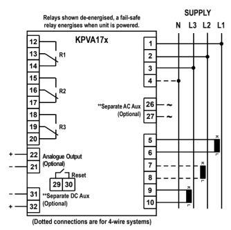
To ensure correct kVAr measurement voltage phase sequence and CT, connections MUST be as shown on connection diagram.
