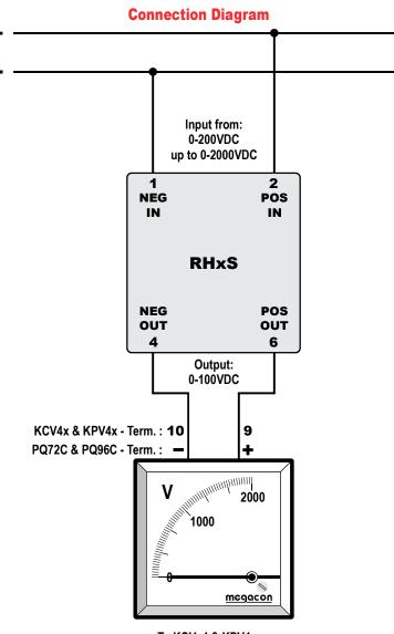
To KCVx4 & KPV4x or PQ72C & PQ96C series Scale: Up to 2000VDC
